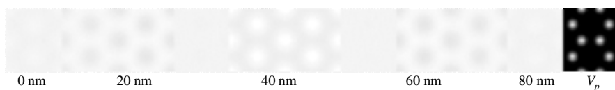
Fig. 3.12. Graphene image simulation for an underfocus series. The contrast is very low ( <0.03 ) and the projected potential is shown on the right-hand side (400 kV, C_s = 1 mm, \delta = 8 nm, \alpha = 0.5 mrad)
